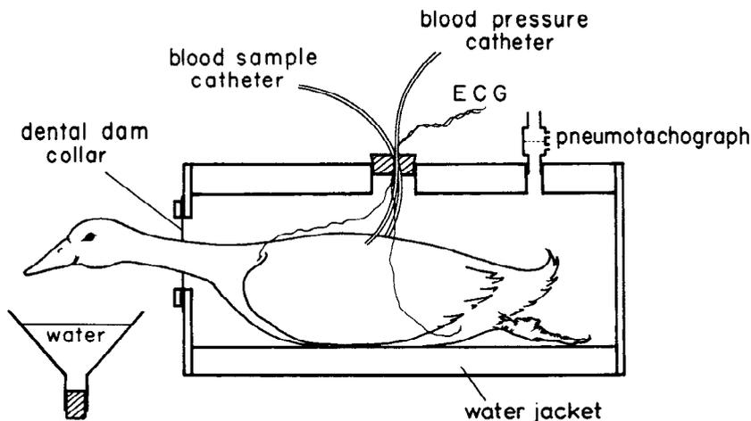
FIG. 1. Diagram of the experimental apparatus. Body plethysmograph is 150 mm (diam) by 500 mm (length) in chamber dimension, and volume of chamber is  $\sim 8.8$  l. ECG, electrocardiogram.
